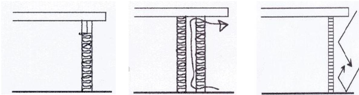
**Figure6: Use Small and High Openings, Double Walls, or Make an External Covering with a Reflective Material.**
